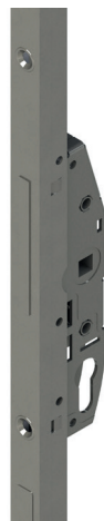
Drive gear with 37.5 mm backset ready for cylinder (80 mm fixing C/C distance)
